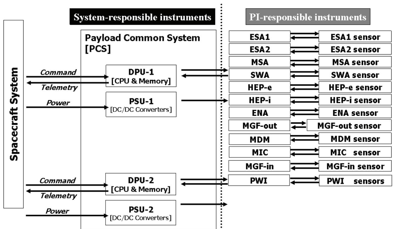
Figure 1. Functional diagram of the MMO model payload package
