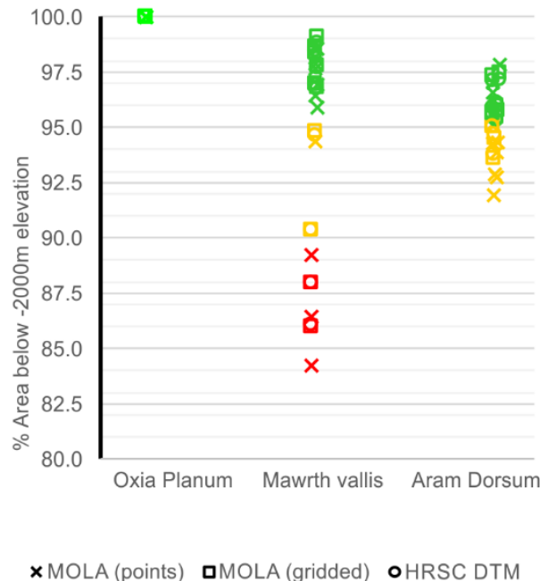
Fig. 2. The percentage area below the -2000m elevation criteria for the 10 sample azimuths at each of the proposed landing sites
