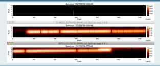
GIBIS Simulation of the above shown target window: GIBIS readout window containing target, background, noise and cosmics (top), GIBIS readout window containing target, background, no noise/ cosmics (middle), GIBIS readout window containing just the background with two overlapping contaminants (bottom).
