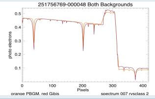
The modelled point source background signal (orange) in comparison to the "true" GIBIS background (red). We see contributions from two contaminants, one is shifted to the right and one is shifted to the left in respect to the target. Around pixel number 300 they overlap by about 40 pixels.
