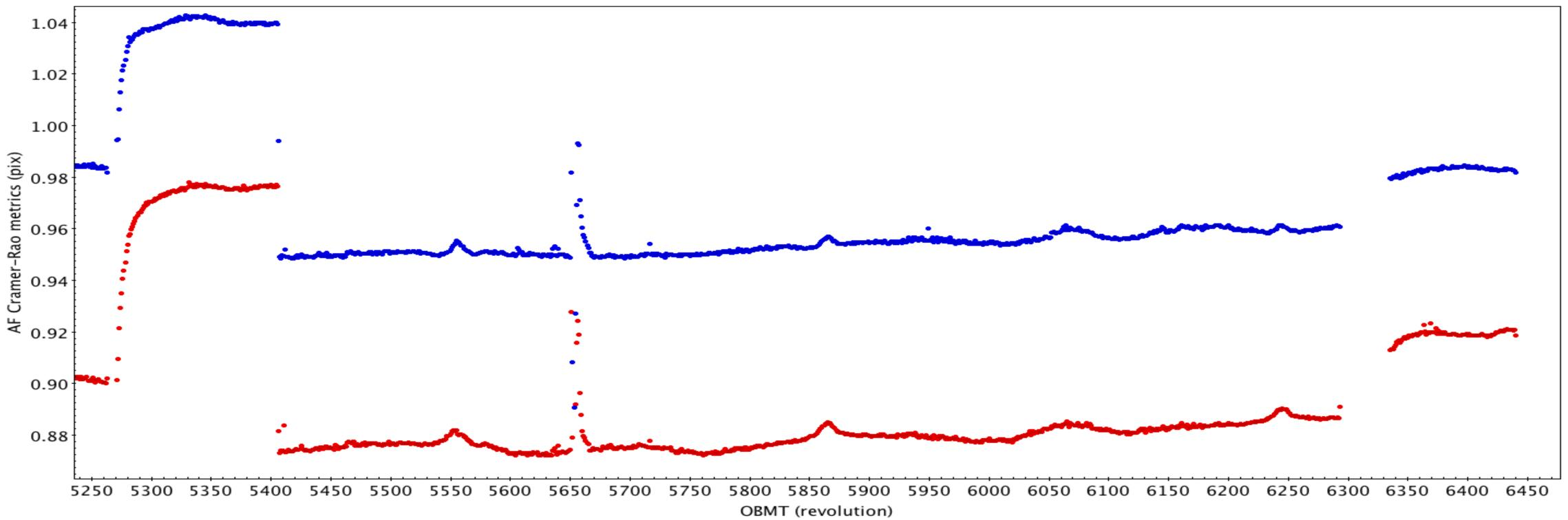
Safe mode 6/17 caused focus degradation of 8.4 and 5.8% respectively to FoV1 & FOV2 => re-focus
