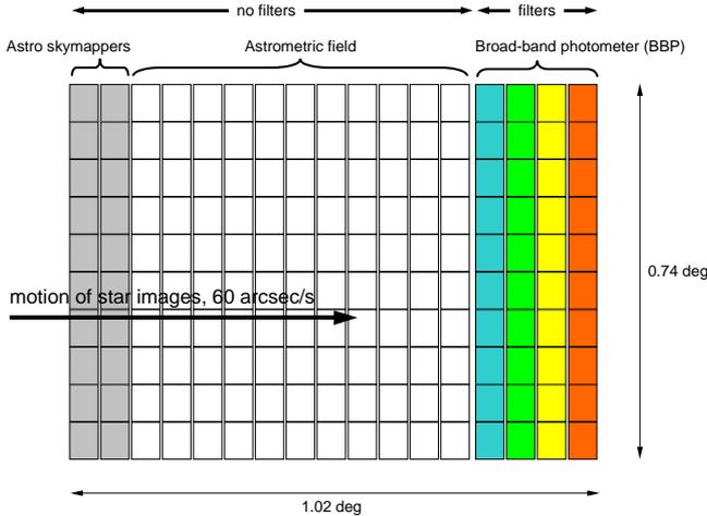
Figure 3. Schematic layout of the astrometric focal plane, comprising 170 identical CCDs in three regions: the sky-mappers and the astrometric field (without filters), and the broad-band photometer with interference filters in front of the CCDs.
