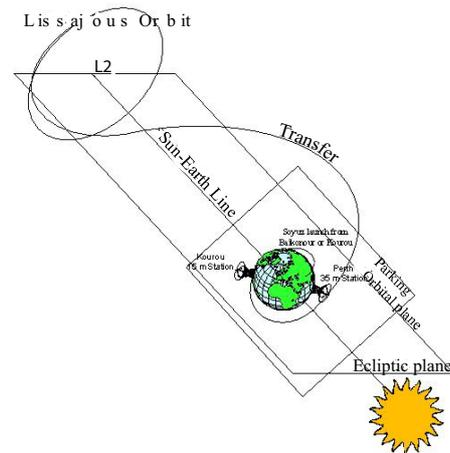
Figure 6. Typical transfer orbit to L2.
