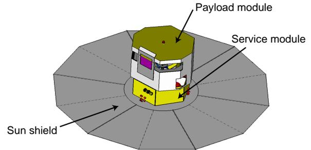
Figure 4. Gaia in orbit – top view.
