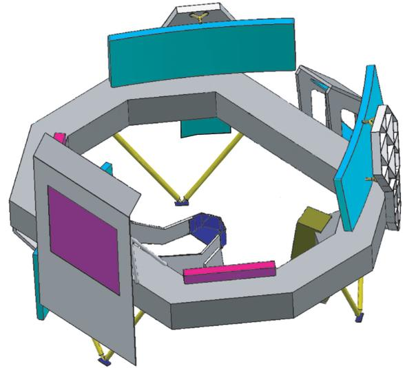
Figure 2. Gaia payload configuration.
