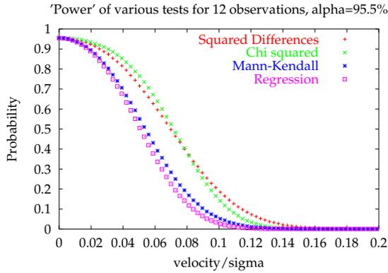
Figure 2. Probability, as a function of actual object velocity, that an object is flagged as stationary. One field crossing, twelve measurements.
