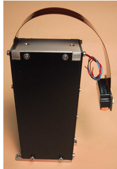
Figure 3. A prototype Proximity Electronics Module (PEM). Courtesy of EADS Astrium and DLR.
