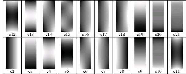
Figure 2. Wavefront maps for the Gram-Schmidt Polynomials  $P_j^{gs}$ ,  $j = 2, \dots, 21$ .  $j = 1$  (piston) is not shown.
