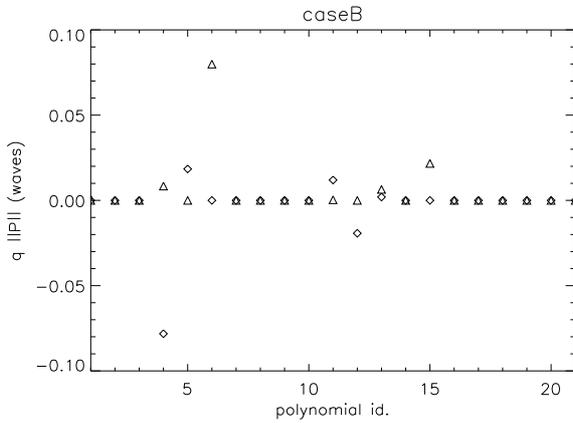
Figure 5. Wavefront  $W_B$ : comparison of the normalised magnitude of each polynomial coefficient for 2-D Legendre (triangles) and Gram-Schmidt (diamonds).
