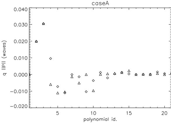
Figure 4. Wavefront  $W_A$ : comparison of the normalised magnitude of each polynomial coefficient for 2-D Legendre (triangles) and Gram-Schmidt (diamonds).
