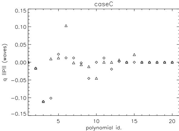
Figure 6. Wavefront  $W_C$ : comparison of the normalised magnitude of each polynomial coefficient for 2-D Legendre (triangles) and Gram-Schmidt (diamonds).
