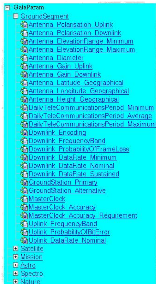
Figure 3. Example of an intermediate step of a browse operation. The ‘Ground Segment’ hierarchical node has been expanded by the user, exposing all associated sub-levels (none in this case) and all individual parameters available at this hierarchical level. A mouse click on any one of these parameters (e.g., ‘Antenna_Diameter’) will return a result window like the one displayed in Figure 2.
