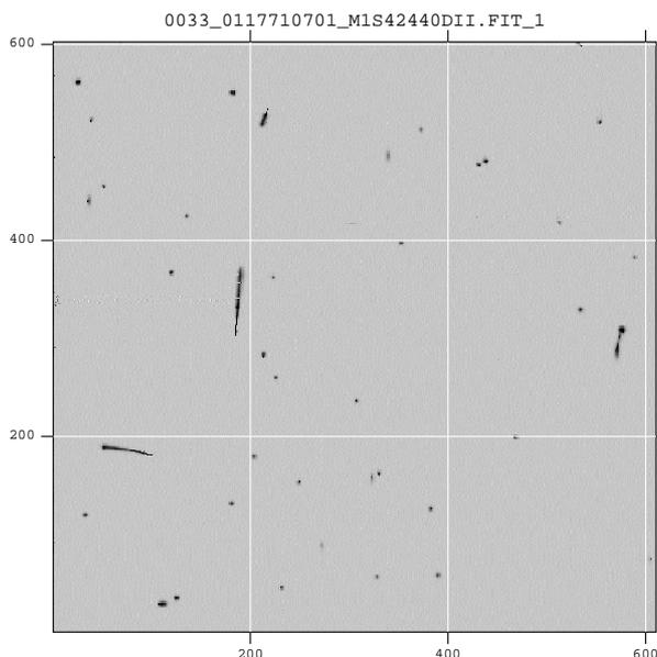
Background particle events (galactic cosmic rays) in an XMM-Newton image. About 60 events were registered on the 2.4 cm×2.4 cm CCD in an integration time of 2.6 s, corresponding to a background rate of 4 events per cm<sup>2</sup> per s.
