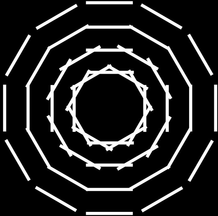
Spacecraft aperture can be 'tiled' with pairs of mirrors to form different baselines
