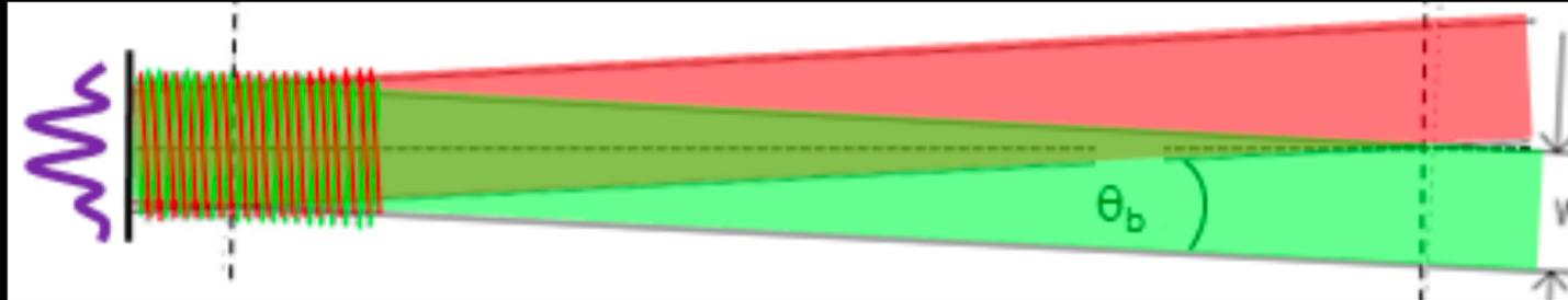
The required focal length  $F = D/\theta_b \approx (4000/\theta_{\mu\text{as}})$  km! Such mirror-detector separations were used by original NASA formation-flyer concepts (Cash, Gendreau, 2003-2010)
