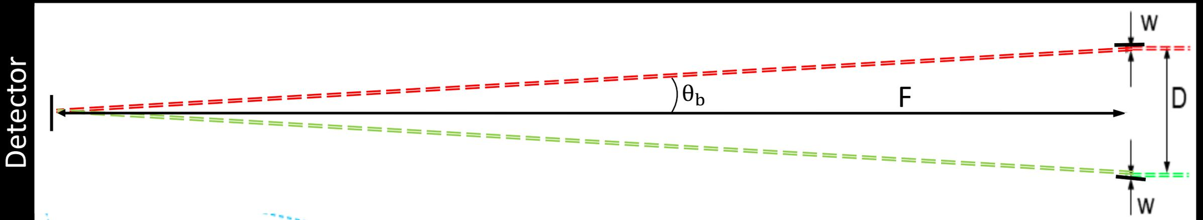
The interferometer can be made **much** more compact (factor 2000!) using a 'telephoto' mirror arrangement (Willingale 2004)
