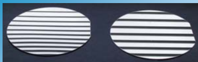
Si wafer (D = 150 mm, 1.3 mm thick) - flat (right) and optically bent (left)
