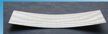
thermally formed Si wafer to test cylinder (R = 150 mm, 72 x 23 x 0.625 mm)
