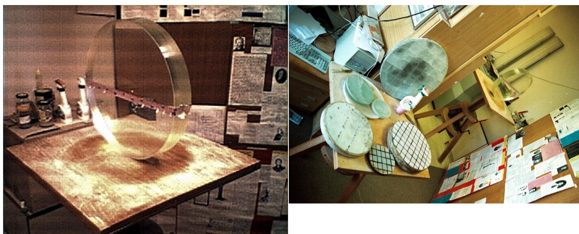
Mirror of D50 telescope in Dr. Polasek's laboratory and tools used to make the mirror.
