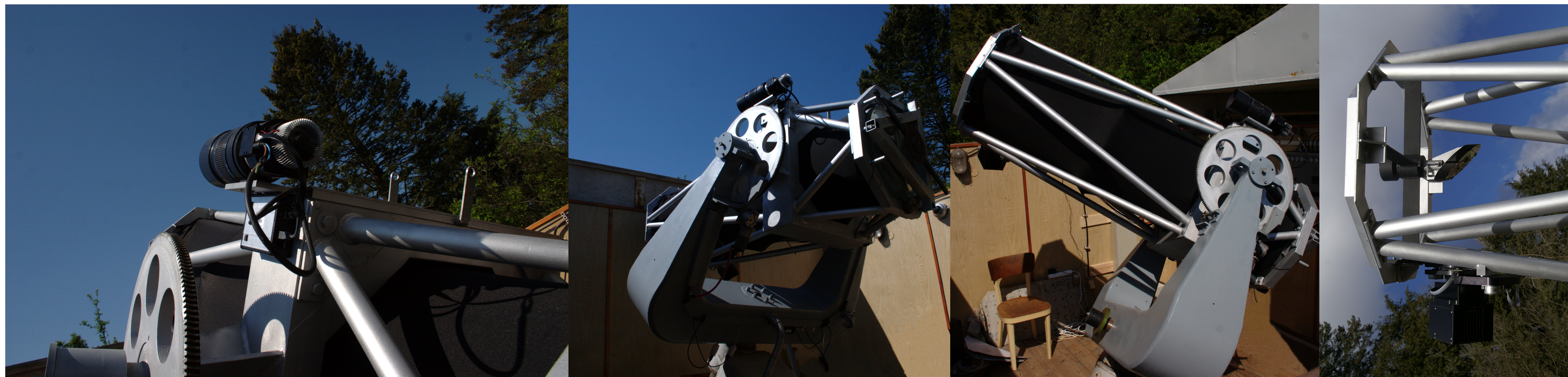
New robotic telescope D50. From left: detail image of wide field camera, image of whole telescope in home position and in random position. In the fourth image there is a detail of secondary mirror and narrow field camera with carousel and focuser without covering robe.
