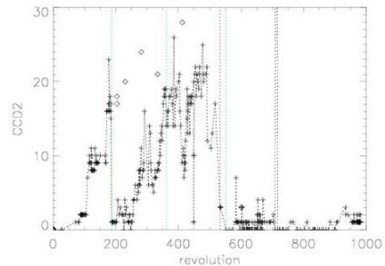
Figure 4 Hot pixel evolution of EPIC-MOS2 CCD2. The diamonds show the absolute number of hot pixels. The crosses show the number of hot pixels that are not yet masked out on board (candidate hot pixels). The green lines indicate an update of the onboard bad pixel table that masks out hot pixels. Note that after the cooling in rev 533 most of the hot pixels have disappeared and the onboard bad pixel table could be relaxed to a few pixels per CCD.
