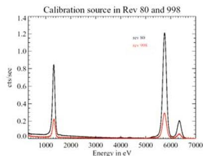
Figure 1: Spectrum of the internal radioactive calibration source in revolution 80 (black) and revolution 998 (red). Note that the calibration source is getting fainter.
