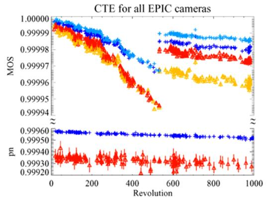
Figure 3: Evolution of the CTE of the EPIC camera CCDs for the energies of the internal calibration source at Mn-K, 5896 eV, (blue crosses) and Al-K, 1486 eV (red triangles). Upper panel: EPIC-MOS, Lower panel EPIC-pn. The different blue and red tones in the upper panel of the figure represent the EPIC-MOS1 (light blue (Mn), orange (Al)) and EPIC-MOS2 (dark blue (Mn), red (Al)). The discontinuity around rev.533 is related to the cooling of the EPIC-MOS cameras
