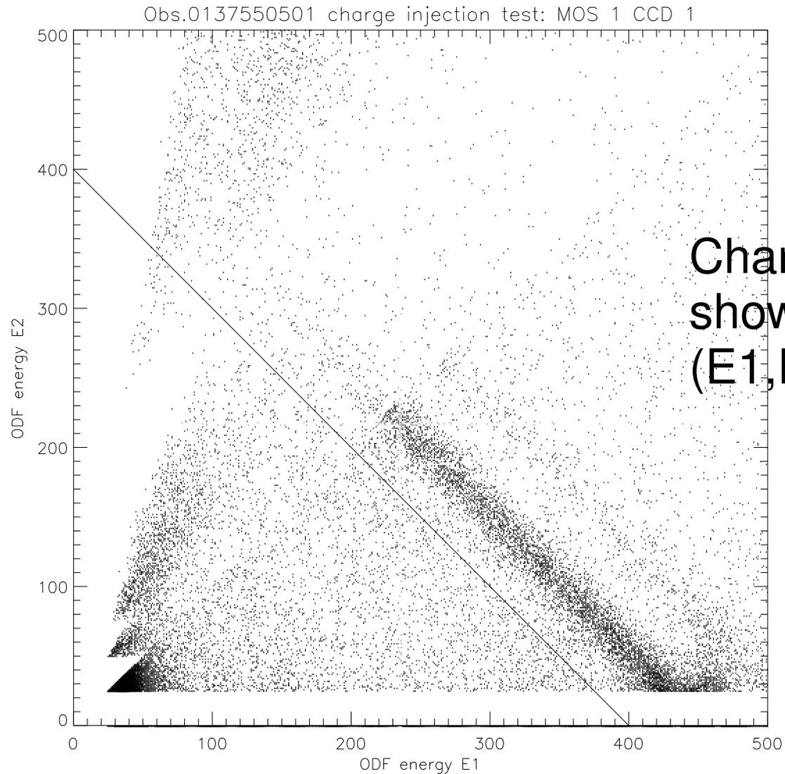
Charge injection test shows no track in (E1, E2)-space.
