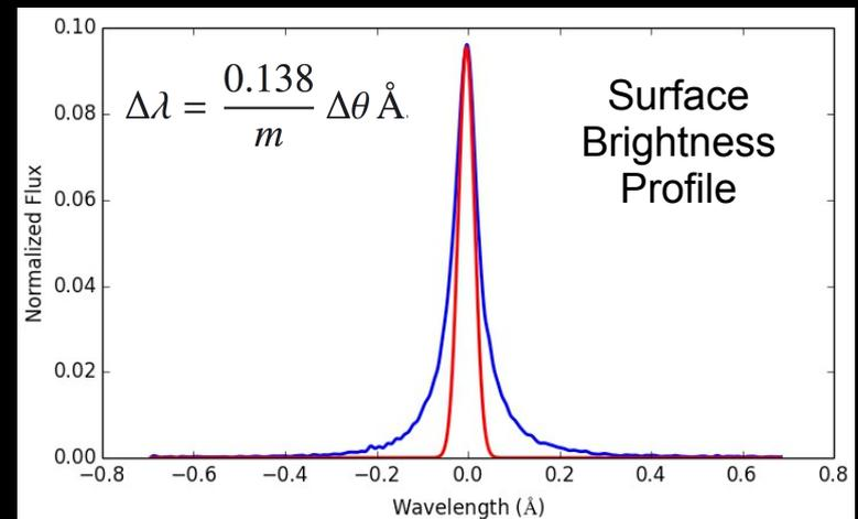
Gaussian fit of line core width
