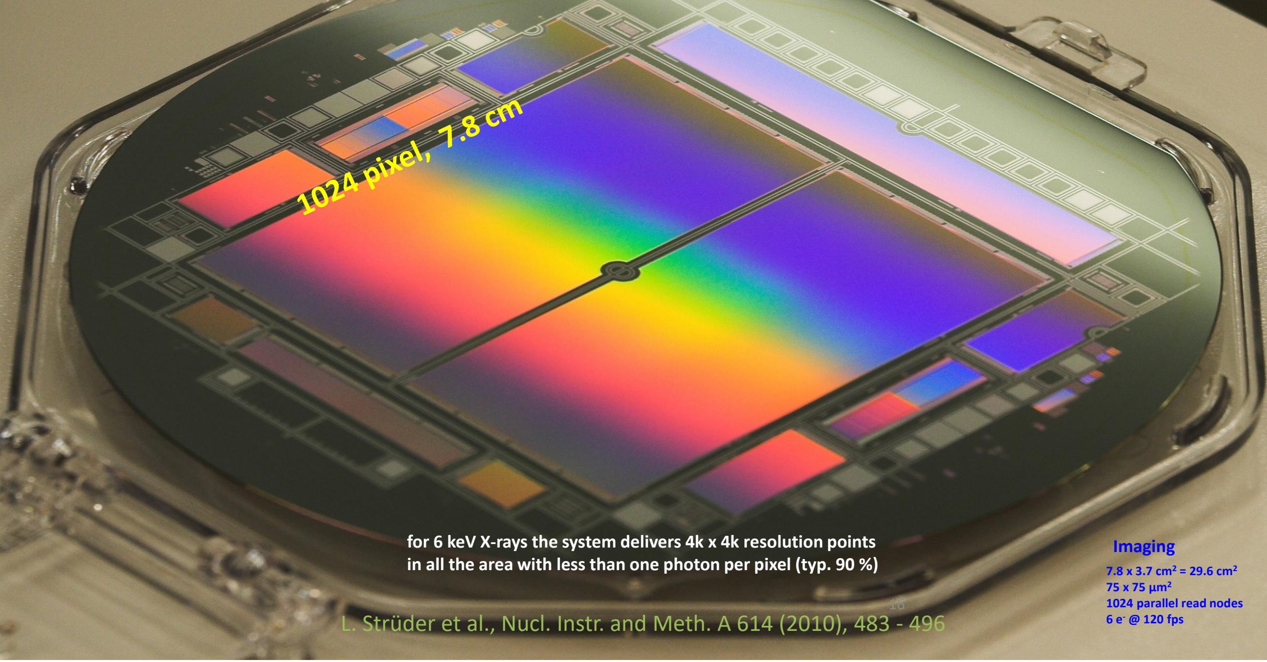
for 6 keV X-rays the system delivers 4k x 4k resolution points
