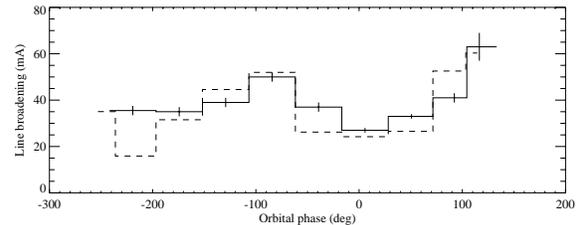
**Fig. 8.** Line broadening of the O VIII Ly $\alpha$  line as a function of orbital phase, for RGS2. Two methods were applied: fit with the line spread function (dashed) and with a double-Gaussian profile (solid).
