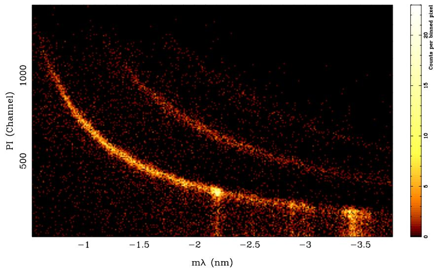
Fig. 5.— Energy-dispersion plot of RGS simulated spectra; LHS from the model detailed in Table 1 and on the RHS from the model detailed in Table 2.
