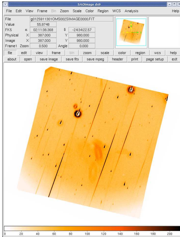
Figure 9: Sky aligned spectral image obtained with the OM UV grism in the field of HD 13499 (the bright object on the mid-right part of the image)
