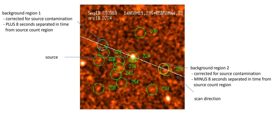
source and background taken in scan direction background corrected for source contamination background with lowest source contamination taken event rates and attitude files checked for scan pathes with detector in OFF mode!
