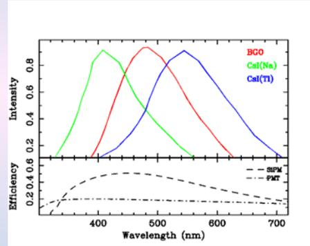
Figure 2: Top panel: the emission spectra of the BGO (red line), CsI(Na)(green line) and CsI(Tl) (blue line). Bottom panel: the PMT and SiPM efficiency.
