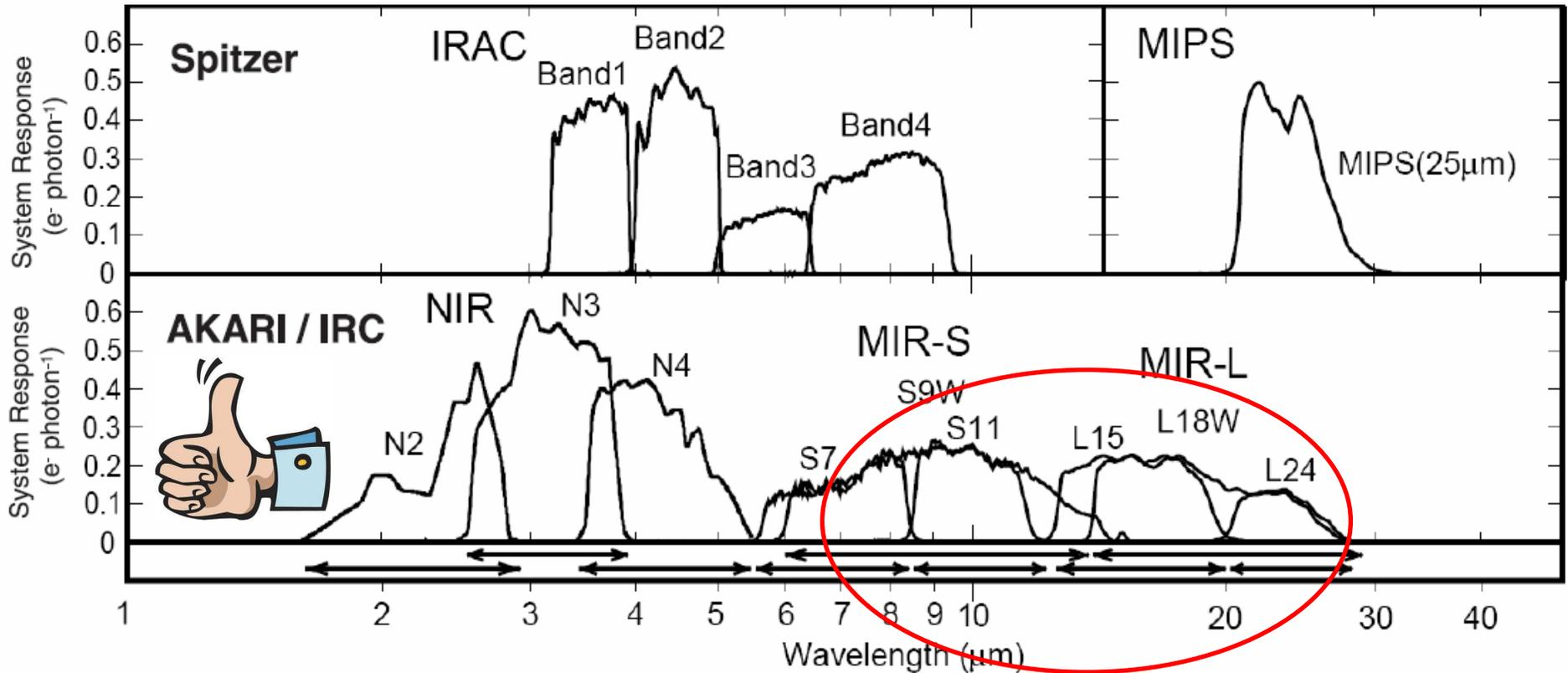
Continuous wavelength coverage from 2-25  $\mu\text{m}$  (9 filters)
