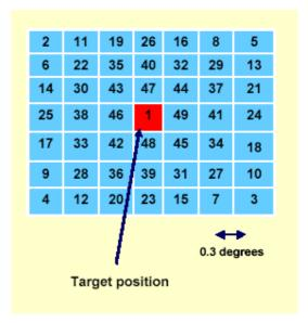
**Figure 1:** 7x7 offset pattern for the central pointing of the nominal 25 point dither pattern.
