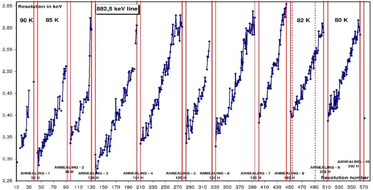
Evolution of SPI's energy resolution at 882.5 keV as a function of time in between the annealing periods.
