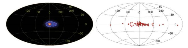
On the left, we see the SPI map of the Galaxy at 511 keV where the asymmetry of the emission from e<sup>+</sup>e<sup>-</sup> annihilation has become apparent after 4 years of deep and regular observations of the central region, and on the right is show the distribution of LMXB detected with INTEGRAL.
