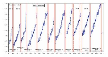
Plot of SPI's energy resolution of the 882.5 keV line as a function of time, showing the effect of the bi-annual annealings.
