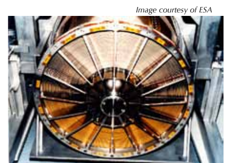
Figure 7: The nested mirrors constituting one of the three telescopes on board XMM-Newton
