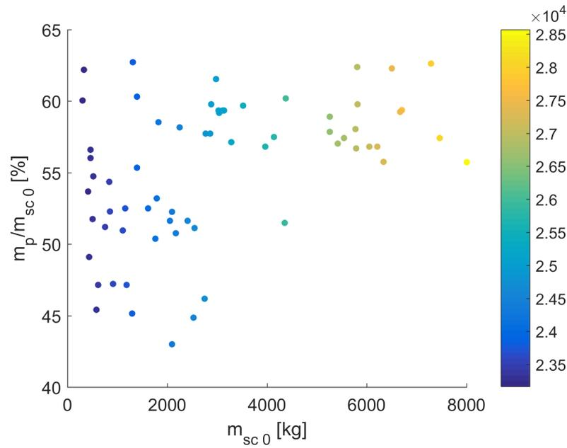
*Spacecraft initial mass vs propellant mass ratio*
