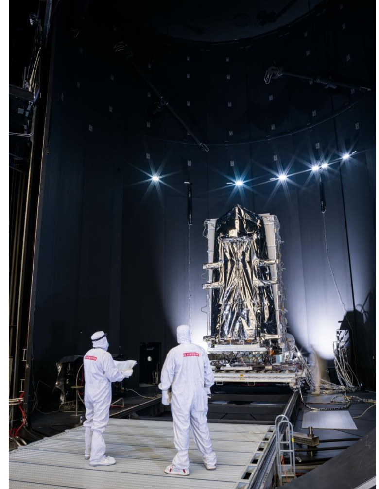
NEO Surveyor instrument enclosure inside the TVAC chamber at NASA Johnson
