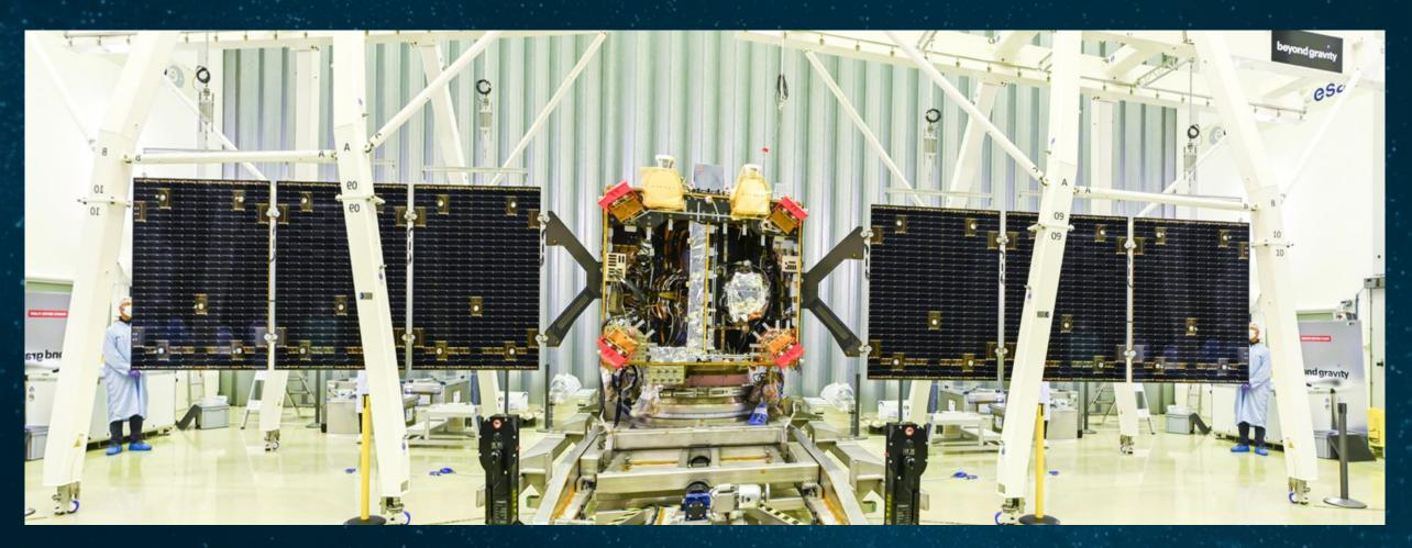
Hera in flight configuration (+z wing mirrored for size purposes)
