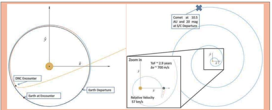
*Fig. 7.2.2. Trajectory for the example mission to C/2001 Q4, in an inertial reference frame (left) and a Suncentred Earth-rotating reference frame (right).*
