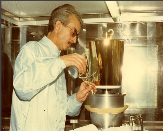
Filling the replication equipment with epoxy at Jobin Yvon
