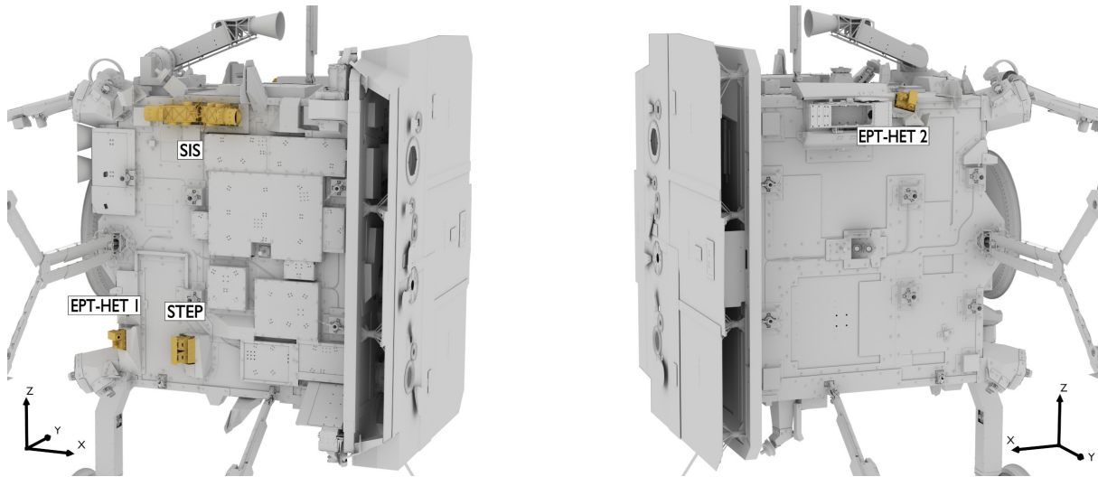
Figure 1: Solar Orbiter spacecraft showing the location of the different EPD sensor units. In the coordinate system of this figure, +X points towards the Sun and the Y and Z complete the orthogonal basis. The left side shows a view of the -Y panel showing the sensors oriented along the mean Parker spiral direction, and the right side shows the view of the +Y panel.
