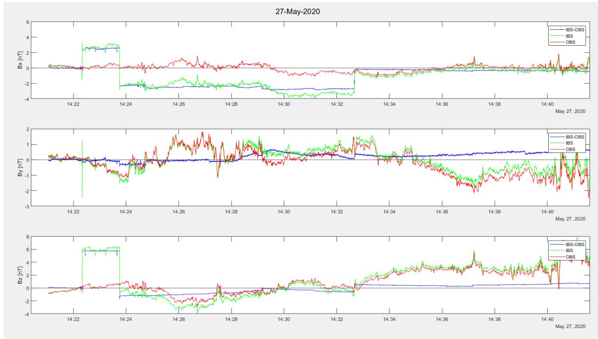
Figure 2-2 Example magnetic field signature from a thruster firing
