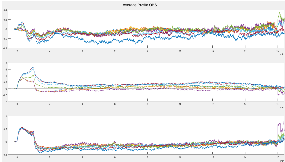
Figure 2-4 OBS heater profile. Each line represents the heater profile averaged over three days. The different colours show the 3 day profile for the days from 16/4 to 23/4 2020.
