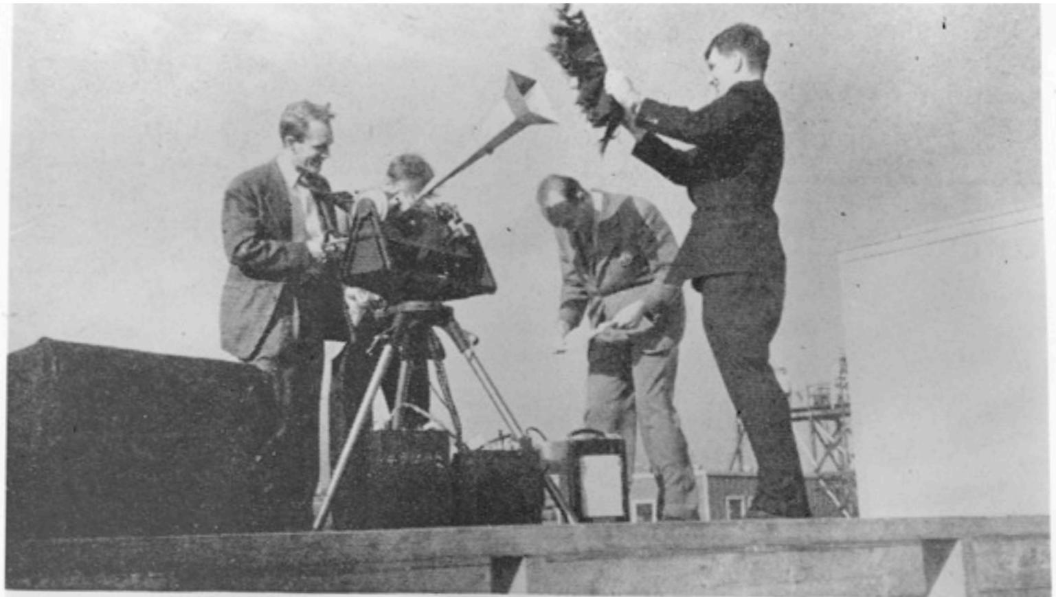
Microwave radiometer, "Shaggy Dog" measured atmosphere's absorption. E. Beringer, R. Kyhl, A. Vane, R. Dicke.
