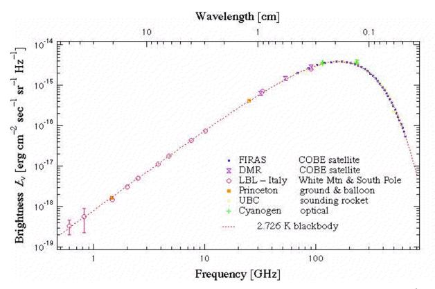
The observations agree: points are measurements; dashed line the expected spectrum
