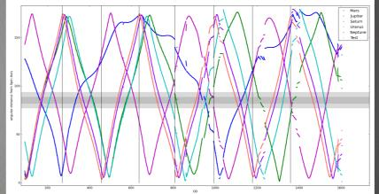
**2. Raw**  $T_{ant}$ , planet antenna temperatures, for each individual radiometer and transit are recovered from calibrated timelines for a known beam response. This is equivalent to apply a linear regression (1)
