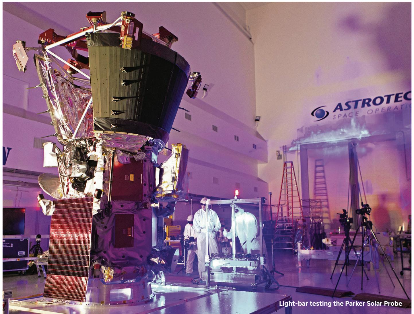
Light-bar testing the Parker Solar Probe
