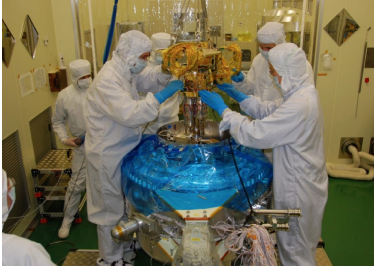
Figure 5. Installation of the flight calorimeter sensor module into the Dewar.
