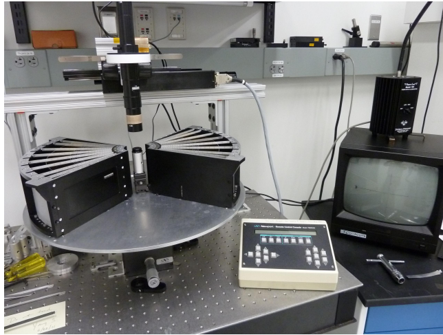
Fig. 4 Alignment setup in polar coordinates. Precision and repeatability of the translation stage was at 1 \mu\text{m} , and wobble of the rotation axis was at 1 \mu\text{rad}
