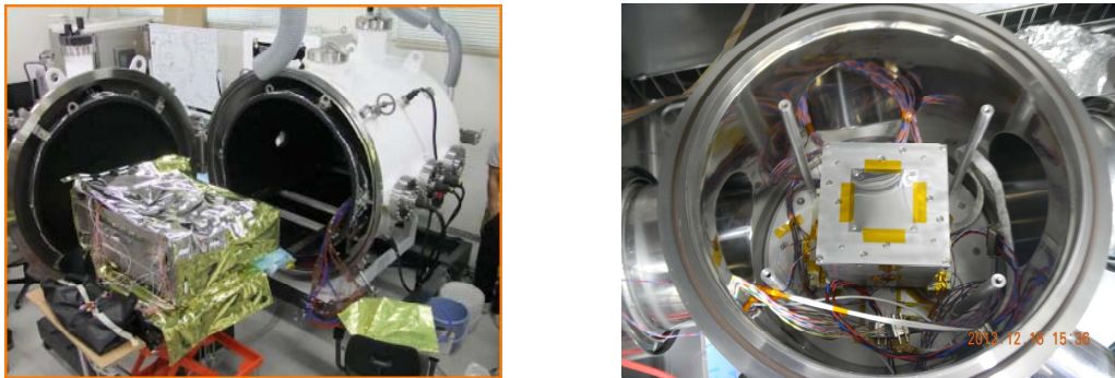
Figure 7. Photos of thermal balance tests in the vacuum of engineering models of SGD-S housing (left) and Compton camera (right).
