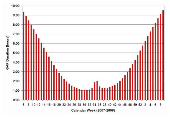
Note the shape of the plot is effectively an inversion of the predicted forcing function, the greater the forcing function, the less time the spacecraft can safely operate without a period of CONSCAN operation.
