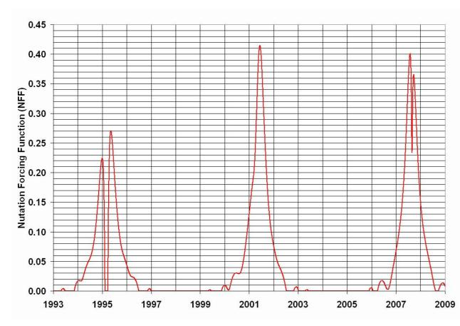
When the SAA is large enough to allow the boom to be illuminated, the Sun provides a continuous thermal input. When the SAA is of sufficient magnitude the driving force for nutation is ever present, meaning the level of nutation can increase. This is modelled by a "Nutation Forcing Function," which is based on heliocentric range and Solar Aspect Angle (i.e. the portion of the boom exposed to sunlight).
