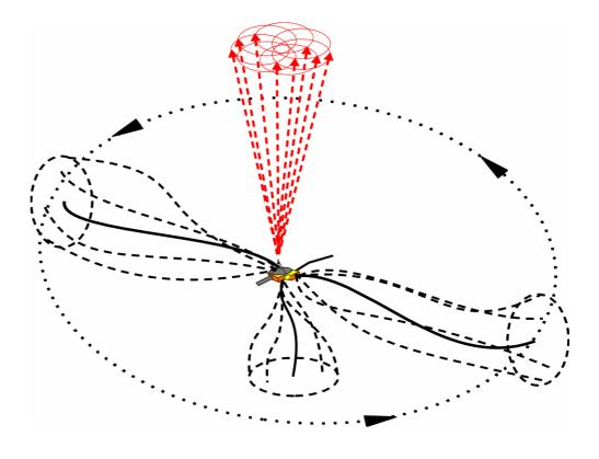
The nutation "rosette", again depicted in red, shows the resulting pattern that the spacecraft telemetry beam would trace if projected into space as the spacecraft nutated. At the very least if nutation were left uncontrolled, it would cause a complete loss of spacecraft engineering and science data.
