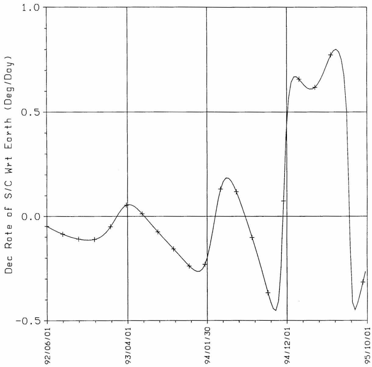
Figure 3-6. Declination Rate of S/C with respect to Earth
