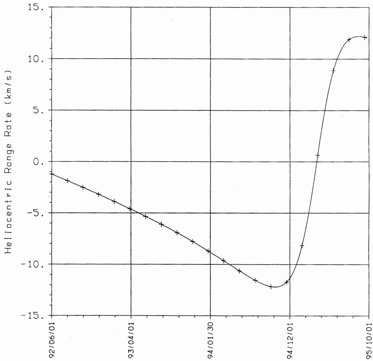
Figure 3-13. Heliocentric Range Rate
