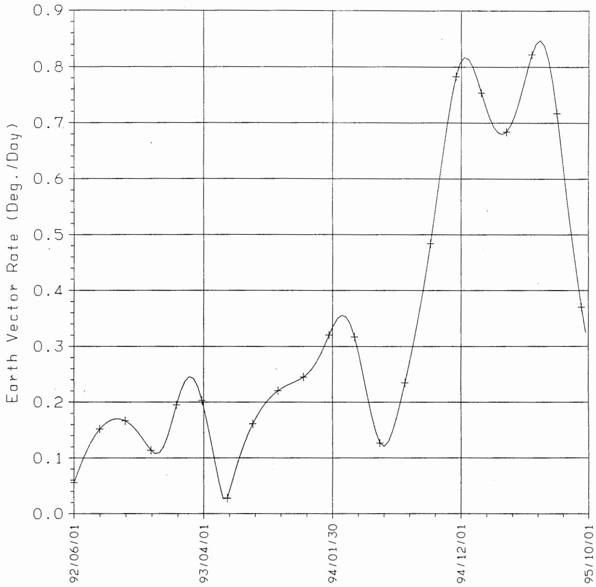
Figure 3-8. Vector Rate of S/C with respect to Earth
