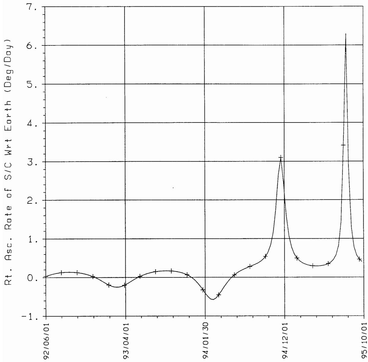
Figure 3-7. Right Ascension Rate of S/C with respect to Earth
