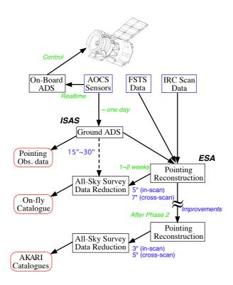
Figure 3.2.2: The outline of the *AKARI* attitude determination for the All-Sky Survey, including time scales and envisioned accuracy improvement. Note that the pointing reconstruction by ESA is not carried out for the pointed observations.
