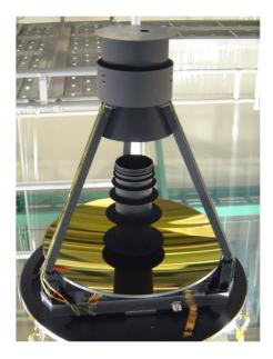
Figure 2.3.4: The AKARI telescope system.
