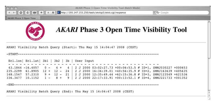
Figure 1.2.2: Results from the Visibility Tool in batch mode. The result shows the total number of allocations possible during Phase 3 of the AKARI mission. Each target is listed by position in Ecliptic coordinates, visibility in Phase 3b1 (2008 Oct. 15 – 2009 Apr. 11 = 179d), Phase 3b2 (2009 Apr. 12 – 2009 Oct. 14 = 186d) and the total visibility in Phase 3 (2008 Oct. 15 – 2009 Oct. 14 = 365d). The original user input is shown on the right.
