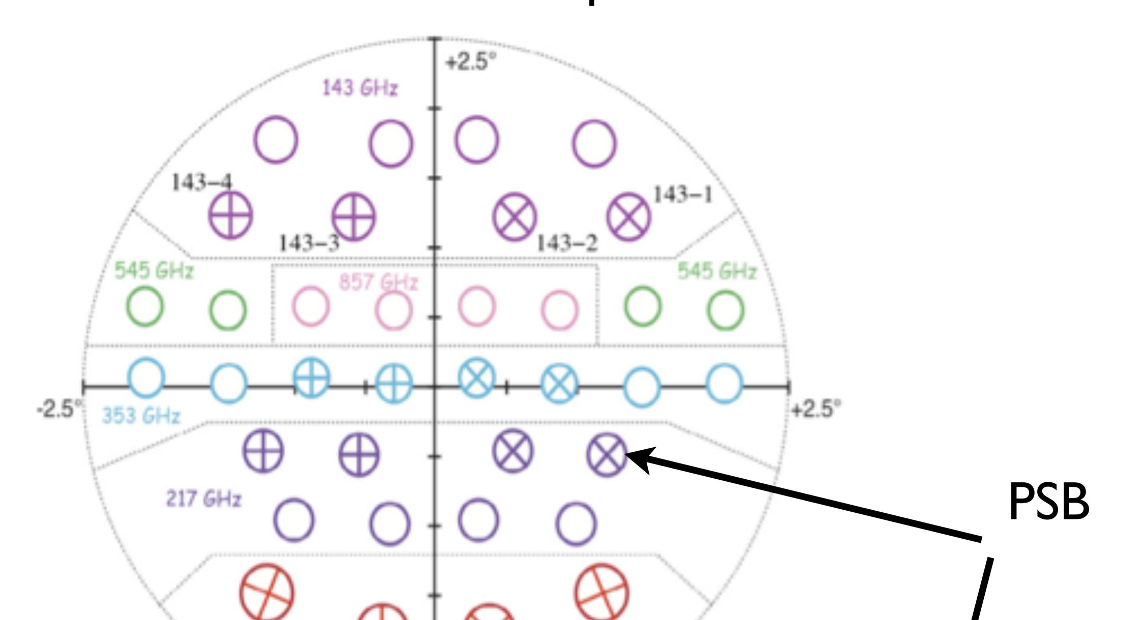
Combination of two pairs of PSB bolometers rotated by  $45^{\circ}$  observing the same sky positions
