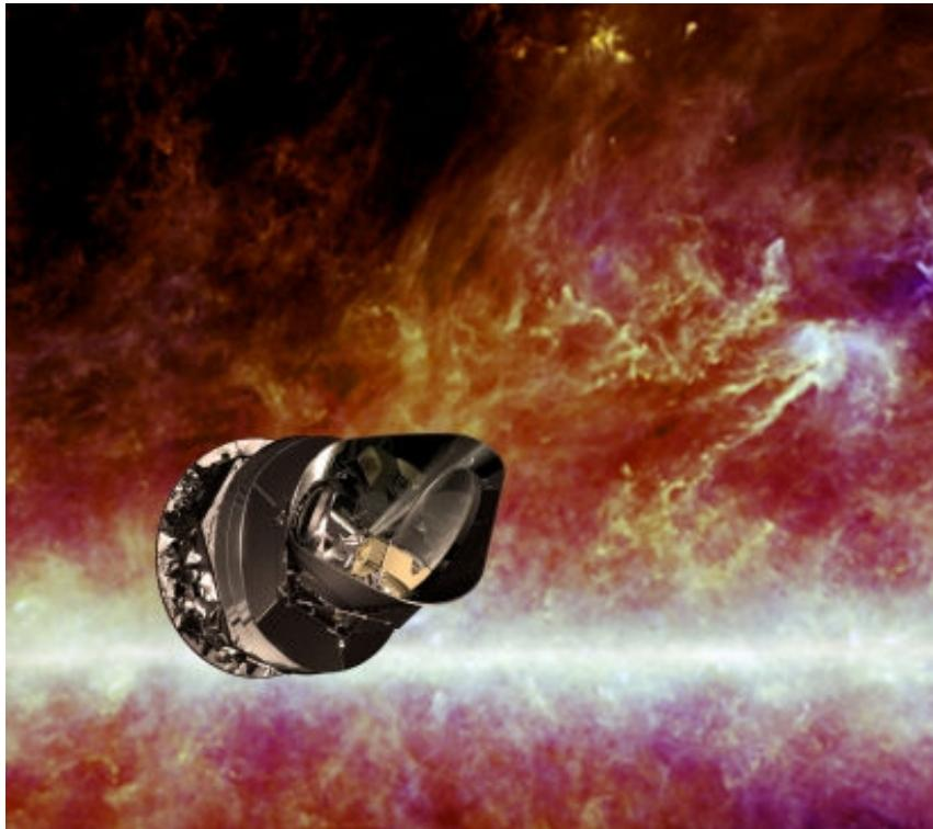
Planck is a third generation space based cosmic microwave background experiment, operating at nine frequencies between 30 and 857 GHz
