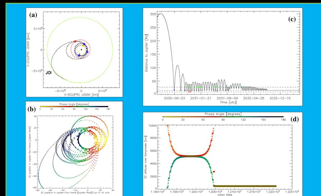
Trajectory: (a) cruise phase – (b) All orbits view from the North - (c) Distances to Jupiter during the Jupiter tour – (d) Distance to Ganymede during the Ganymede phase (elliptical orbits, 5000/500 km circular orbits).
