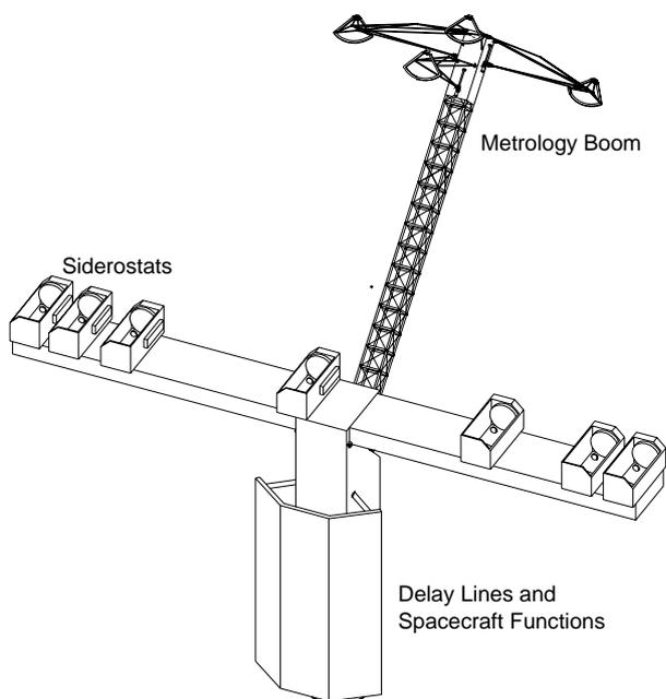
Figure 1. The SIM spacecraft based on the OSI architecture. Six siderostats operate as three pairs of Michelson interferometers. The seventh siderostat is a spare and fills in missing baselines for synthesis imaging.
