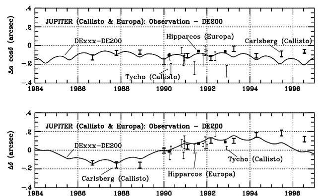
Figure 3. Comparison of the observation positions of Jupiter with DE200 and DExxx ephemerides (upper, right ascension; lower, declination). The Hipparcos normal points derived from observations of Europa are shown as filled squares. Individual Tycho positions derived from observations of Callisto are plotted as light error bars. The opposition means derived from Carlsberg Meridian Telescope observations of Callisto are plotted as heavy error bars.
