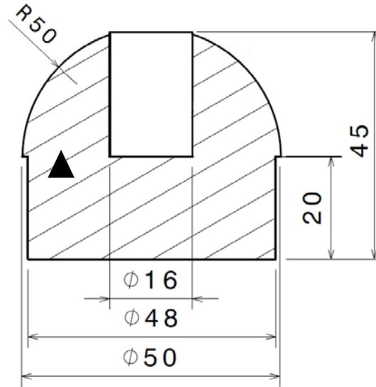
Figure 6. Hemispheric holder configuration
